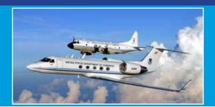
violent updrafts and downdrafts before entering the relative calm of the storm's eye, NOAA's two Lockheed WP-3D Orion four-engine turboprop aircraft, affectionately nicknamed "Kermit" (N42RF) and "Miss Piggy" (N43RF), probe every wind and pressure change, repeating the often grueling experience again and again during the course of an 8-10 hour mission.
